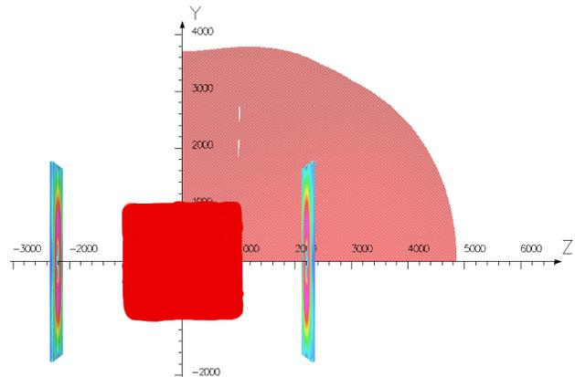
Figure 2: 3D simulations of the solenoid's magnetic field with the latest magnetic shielding design. In addition, the envelope of the 5 G limit around the ISS magnet is shown in light red.
