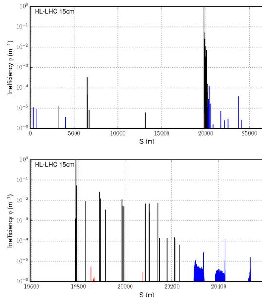
Figure 3: Loss maps for HL-LHC 15cm squeezed optics, whole ring above and IR7 below. Collimator, warm and cold losses are shown in black, red and blue respectively.
