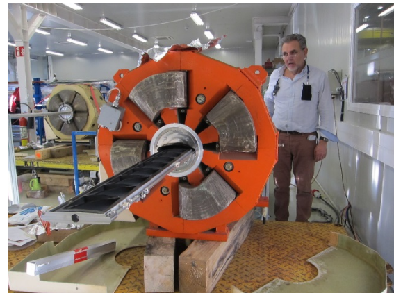
Figure 3: QF type cathode inserted in a SSS magnet with elliptical vacuum chamber.
