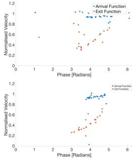
Figure 7: Arrival and exit velocities of electrons, at a beam radius of a) on-axis, and b) 5.2 mm, simulated by MAGIC2-D.
