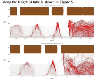
Figure 4: Electron bunch profile in a) the optimised case, and b) unstable klystron, simulated by MAGIC2-D.
