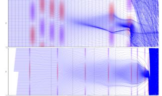
Figure 1: Electron phase profile of a) the SLAC 5045 klystron, and b) a klystron employing the Core Oscillation Method (COM).
