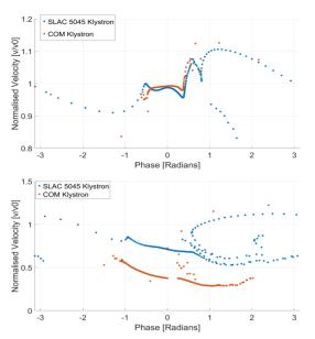
Figure 2: Comparison of arrival functions a) entering, and b) exiting the output cavity of the SLAC 5045 and a COM klystron.
