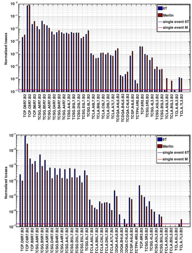
Figure 3: Inelastic (above) and single diffractive (below) losses at named collimators in MERLIN and SixTrack.
