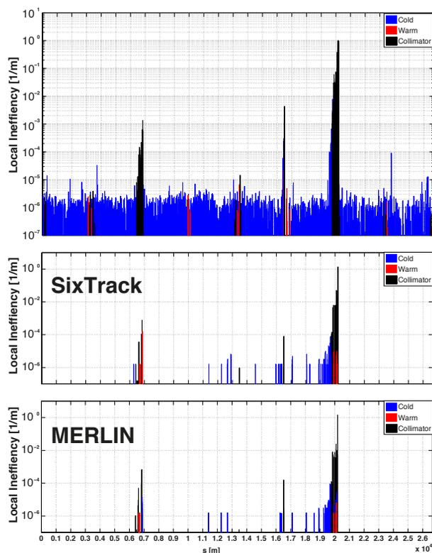
Figure 1: Beam loss distribution around the LHC. On top losses measured with BLMs from a qualification loss map of the betatron collimation system on September 2015 compared to simulations performed with SixTrack (centre) and MERLIN (bottom).
