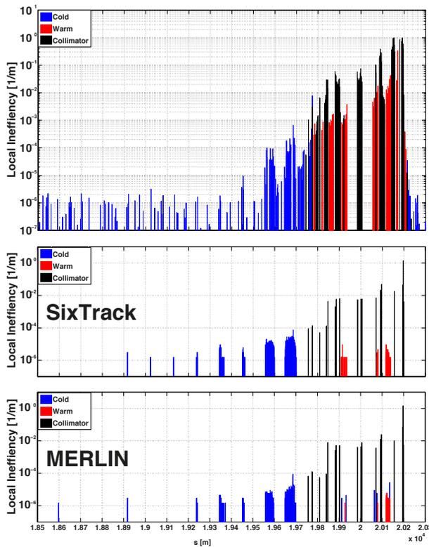
Figure 2: Loss locations in IR 7 (zoom of Fig. 1) from measurement (top), SixTrack (centre) and MERLIN (bottom).
