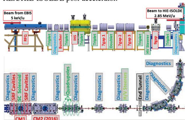
Fig. 1: Layout of the post-accelerator and one of the HEBT lines (REX on the top, HIE-ISOLDE on the bottom). RF structures labelled in red, diagnostic boxes in blue and magnetic elements in green.
