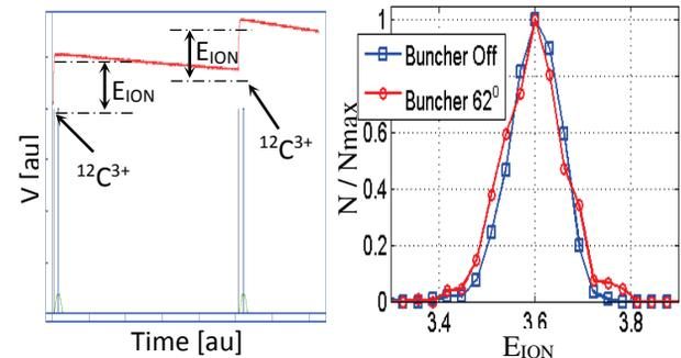
Fig. 3: On the left in red, typical signal when ions impact in the Si detector. Height of the signal proportional to the energy of the ion ( $E_{ION}$ ). On the right, energy spectrum of a  $^{12}\text{C}^{3+}$  beam with the buncher off and with the buncher set at its zero-crossing phase. Note that the measured energy spread does not change since it is dominated by the resolution of the detector.
