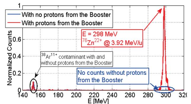
Fig. 4: Energy spectrum of the beam delivered to the Miniball experimental station. RIB of interest ( $^{76}\text{Zn}^{22+}$ ) and EBIS contaminant ( $^{38}\text{Ar}^{11+}$ ) in red. Only the contaminant is visible when the primary proton beam from the PSB is stopped (in blue).
