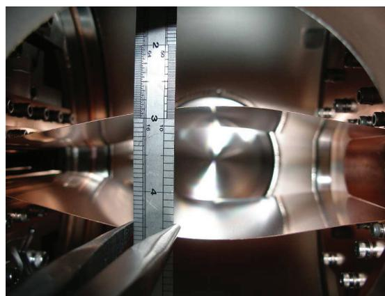
Figure 2: Transition taper view at 6mm gap on IVU05.
