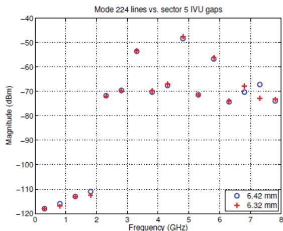
Figure 6: IVU 5 mode 224 resonance line strengths at different harmonics when on-resonance (blue dot) and off-resonance (red cross).
