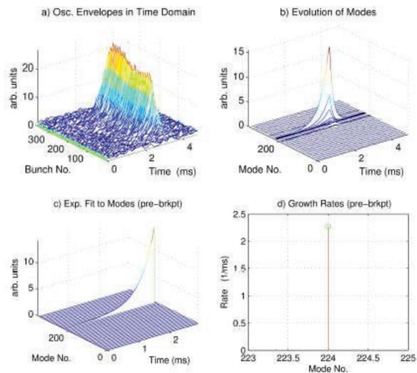
Figure 3: Grow/damp measurements using Dimtel transverse feedback system.
