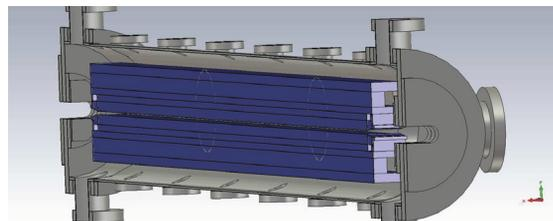
Figure 1: Geometry of the 2m IVU, in cutaway view. Transition tapers and feed-throughs are not shown.
