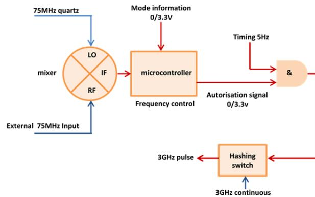
Figure 4: Frequency drift security system.
