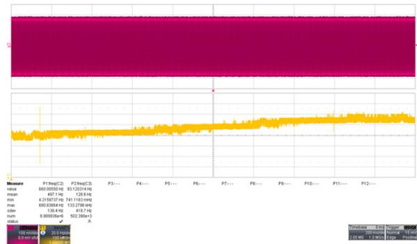
Figure 3: Frequency shifting of Laserix cavity oscillator versus time.
