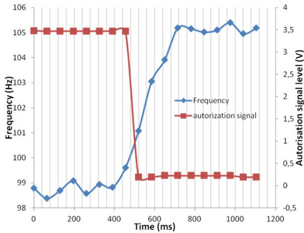
Figure 5: Response time of the frequency drift security.
