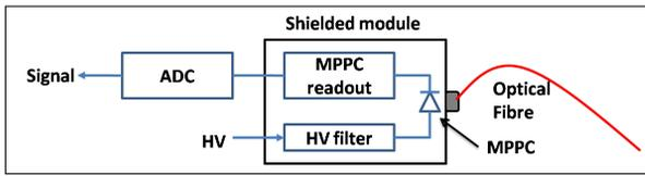
Figure 1: Schematic layout of the photosensor electronics.
