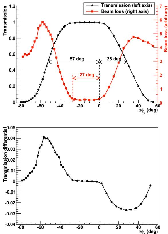
Figure 3: (Top) Experimental result of phase scan. The black line with filled circles is the transmission result (left axis), and red line is the sum of all BLM signals between DTL to SDTL sections. (Bottom) The differential of the transmission of the top figure.
