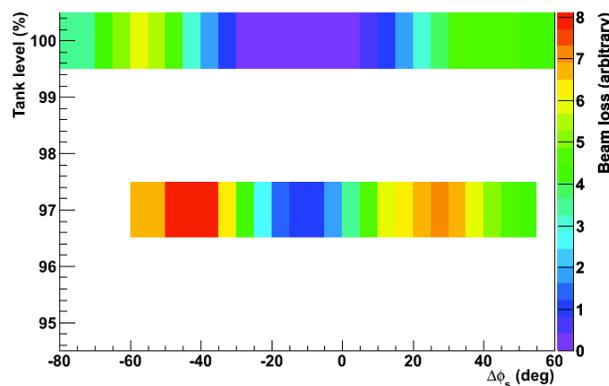
Figure 5: The BLM data of the tank level scan. The beam loss becomes larger as warm colors.
