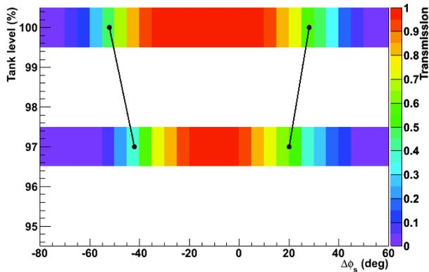
Figure 4: The transmission data of the tank level scan. We measured the transmission at the tank level of 100 % and 97 %. The black lines with filled circle shows the acceptance edge of each tank level.
