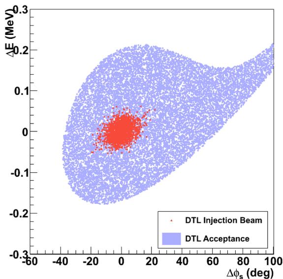
Figure 1: Longitudinal acceptance at the DTL entrance (blue points). Design beam distribution at the DTL entrance (red points) is also shown for comparison.
