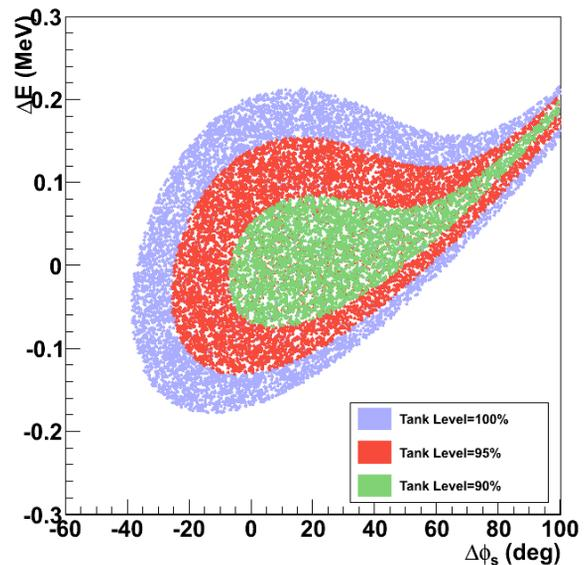
Figure 2: The longitudinal acceptance at the DTL entrance with the tank level of the 1<sup>st</sup> DTL cavity scaled to 100 % (blue points), 95 % (red points) and 90 % (green points) of the design value, respectively.
