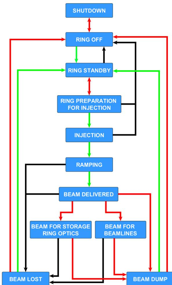
Figure 1: Schematic diagram presents all states of the state machine with set transitions. The color of the connection/transition: red - transition triggered by an operator or watchdog, green - transitions is triggered automatically after fulfilling specified conditions, black - transition has been made automatically in a case of lock comes from the PSS or MPS system [1].
