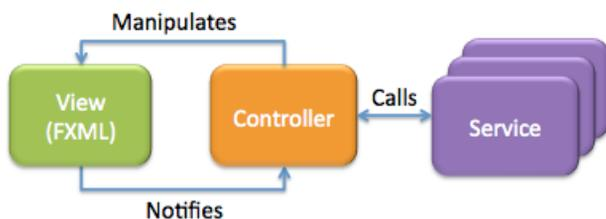
Figure 1: Simple variant of a Supervising Controller
