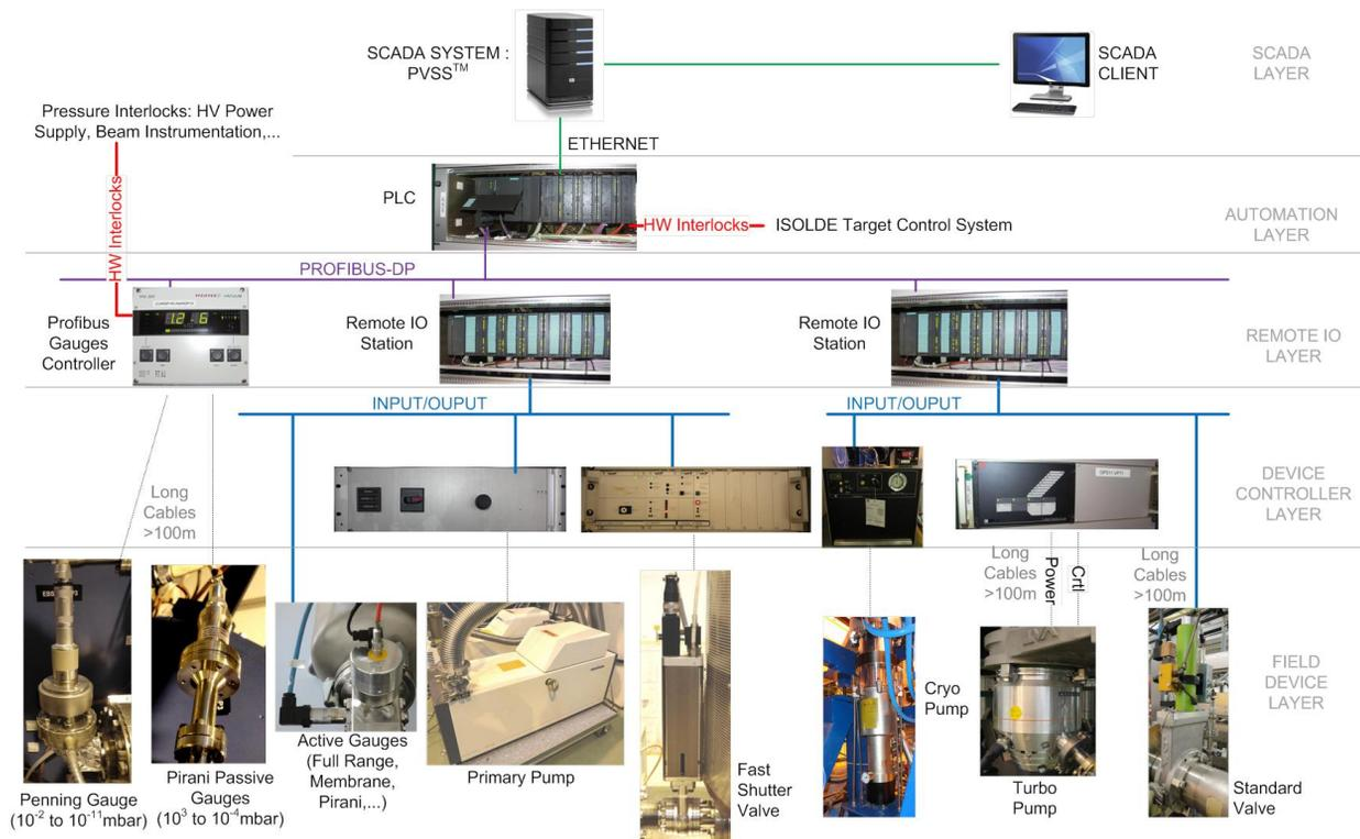
Figure 4: Hardware Architecture.
