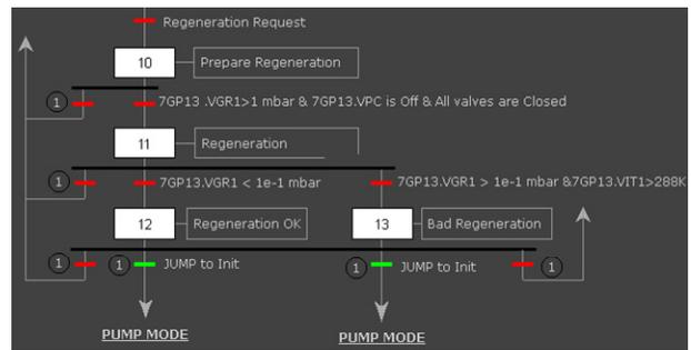
Figure 5: Part of a cryogenic pump process Grafcet (SCADA Panel).
