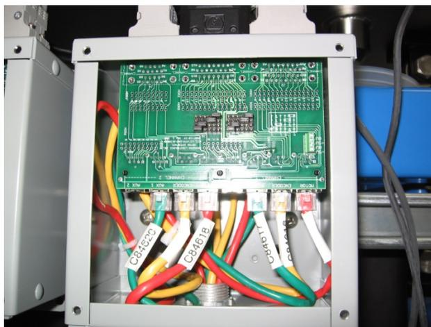
Figure 2: CLS motor control interface board.
