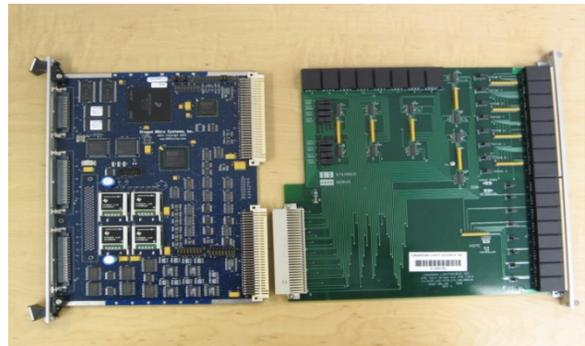
Figure 1: Control card and break out board.
