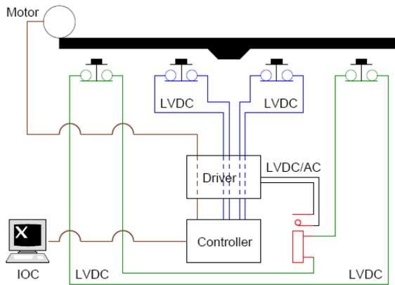
Figure 3: Independent limit switch scheme.
