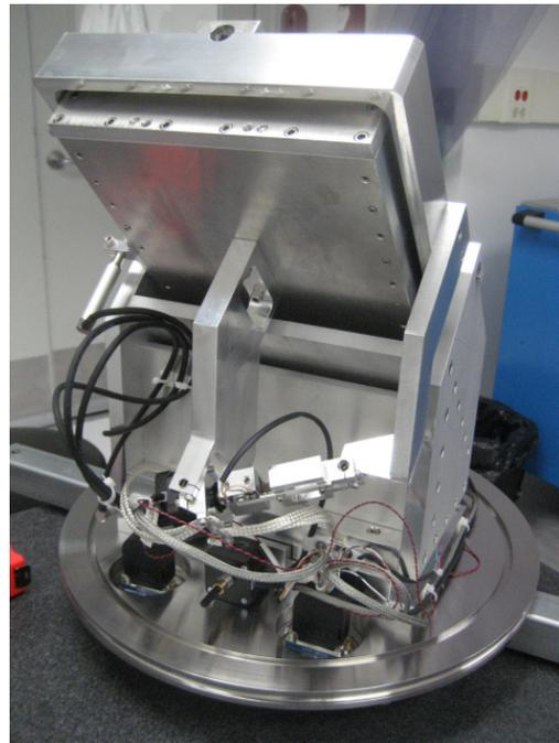
Figure 4: Far-IR mirror mount with motors.
