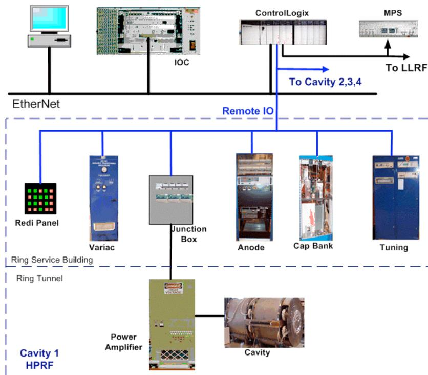
Figure 1: SNS Ring HPRF Control System Layout
