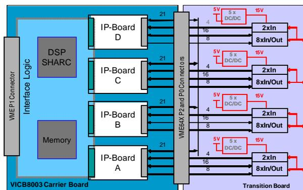
Figure 2 : HYTEC carrierboard with DSP
