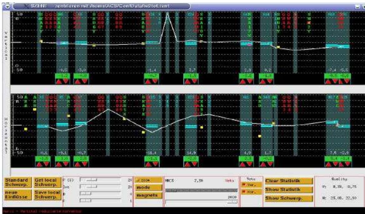
Figure 4: Automated centering utility showing in the upper part, the vertical beam position and in the lower part the horizontal beam positions
