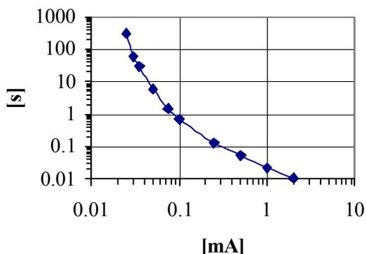
Figure 1: Time for melting steel at E=590 MeV for a beam with  $\sigma = 1\text{mm}$  [1]
