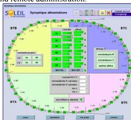
Figure 3: General supervisory application for Booster Control
