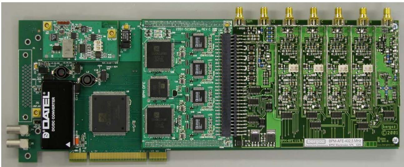
Figure 2: The BPM system PCI card showing the clock multiplier (top left), DFE (center) and AFE (right).
