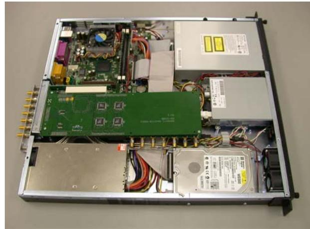
Figure 4: SNS BPM system in 1U, rack-mount PC
