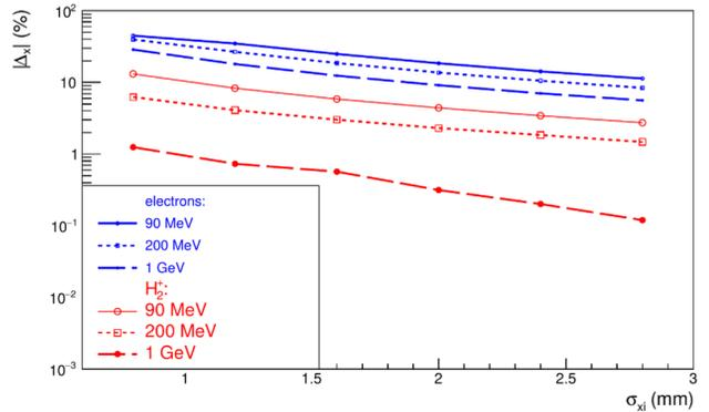
Figure 1: Space charge effects (given as deviation between the beam width input in the simulations and the one obtained by running the code) for different  $\sigma_{xi}$  (i.e. input  $\sigma_x$ ) and incident beam energies when  $\sigma_y = \sigma_z = 2$  mm and  $\mathbf{E} = E_y = 300$  kV/m.
