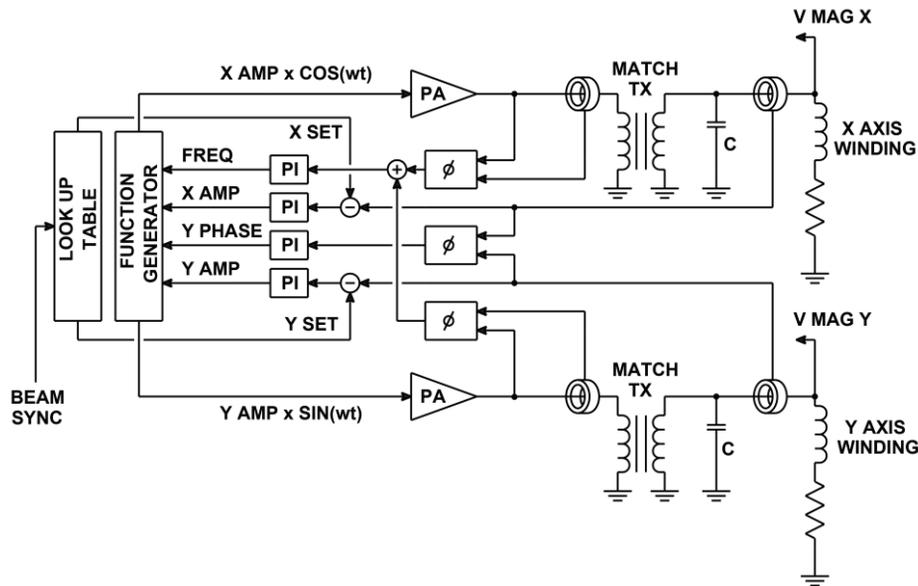
Figure 3: Schematic of the power amplifier control that is implemented by software.
