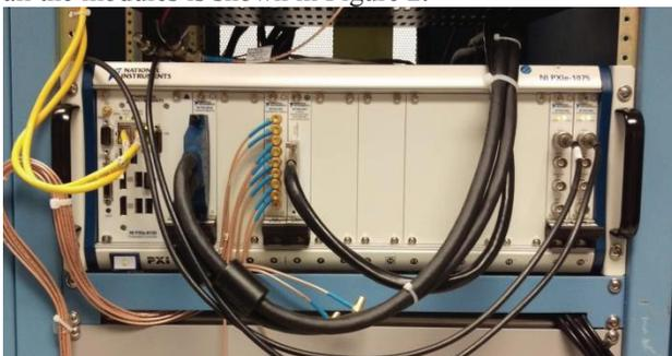
Figure 2: The National Instruments PXIe platform with 18-slot chassis and I/O modules.
