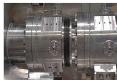
Figure 2: Picture of two of the DBPM’s mounted in the Diagnostics Plate.
