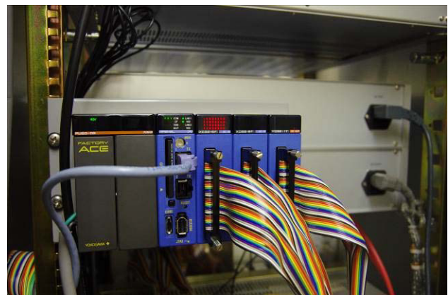
Figure 5: Yokogawa FA-M3 system to read interlock status and to reset the latched interlock. From left, power supply unit, CPU unit, two 32-bit TLL input unit and 32-bit TTL output unit.
