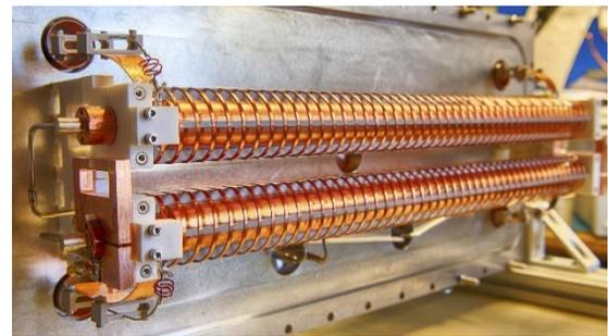
Figure 3: Photo of the fully assembled 200 Ohm kicker's two-helix structure.
