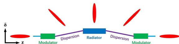
Figure 1: One super-period of longitudinal strong focusing.
