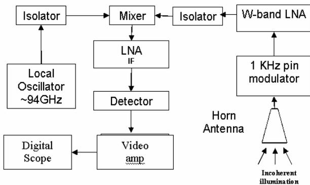
Figure 5: Schematic of the wide band mm-wave sensor.
