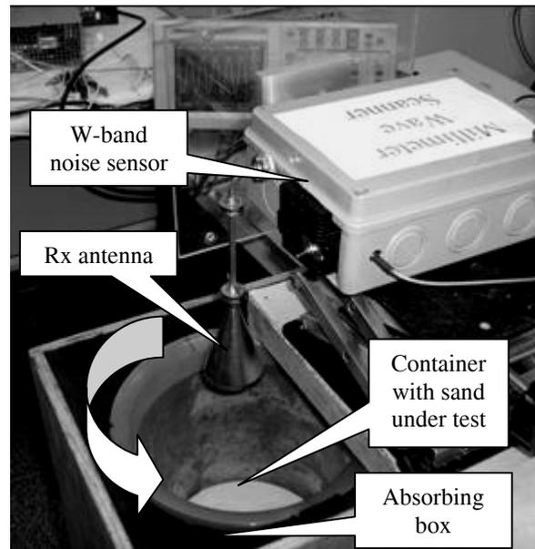
Figure 6: The general view of the setup used for quasi-noise characterization of building materials.
