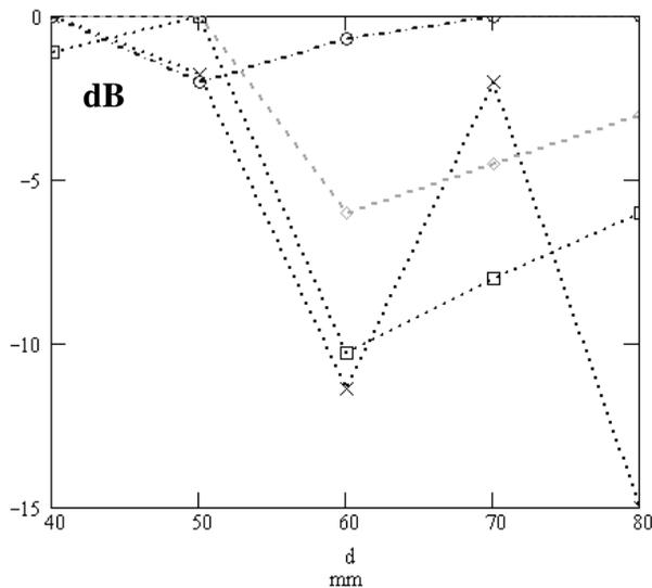
Figure 8: Measured attenuation for coherent illumination at 100 GHz as a function of sand's layer thickness for the four angular position of container: 000 - 0 deg, xxx - 90 deg,  $\diamond \diamond \diamond$  - 180 deg and  $\square \square \square$  - 270 deg.
