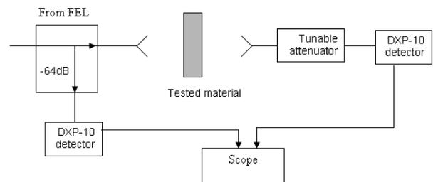
Figure 2: The block-diagram of the experimental setup.
