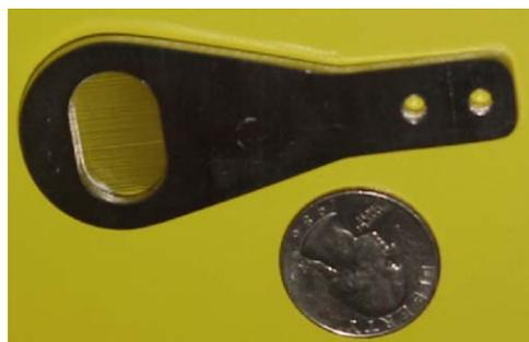
Figure 3. Photograph of the wire target for adjustable microbunch beam generation.
