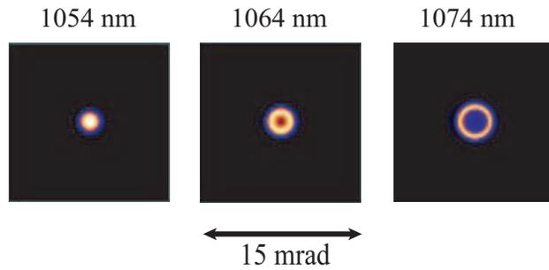
Figure 7: GENESIS simulation of the far-field angular distribution patterns of the seeded FEL for different values of detuning (1064 nm is the nominal wavelength).
