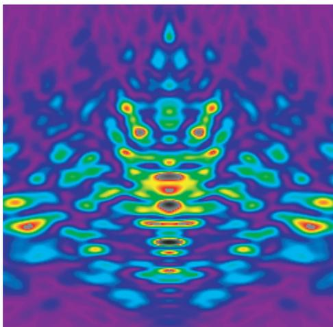
Figure 6: Spectrogram (with frequency along the vertical axis and time delay along the horizontal) of the expected radiation from the VISA II experiment. Further processing of this spectrogram has yielded the longitudinal profile of the pulse used in simulations.
