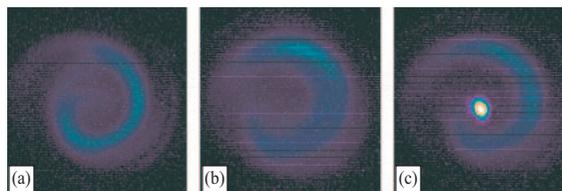
Figure 5: Far-field angular distribution profiles display an atypical spirality and helicity (a,b); superimposed with a reference alignment laser (c).
