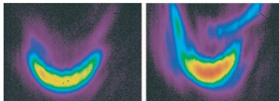
Figure 4: The parabolic structure (left) is evident in the images from the double differential spectrometer, where the angle is represented along the horizontal axis and the frequency along the vertical. Richer structures have also been observed (right).
