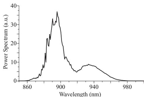
Figure 3: SASE FEL power spectrum obtained from GENESIS. The large bandwidth and the double hump feature observed in measurements were reproduced with simulations.
