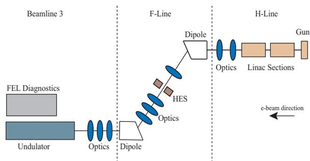
Figure 1: Layout of the ATF beam transport (not to scale). The VISA undulator is located along Beamline 3 after the 20 degree dogleg.
