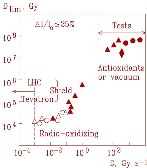
Figure 1: Radiation stability of polymerconcrete (see Table 2 for the legend).
