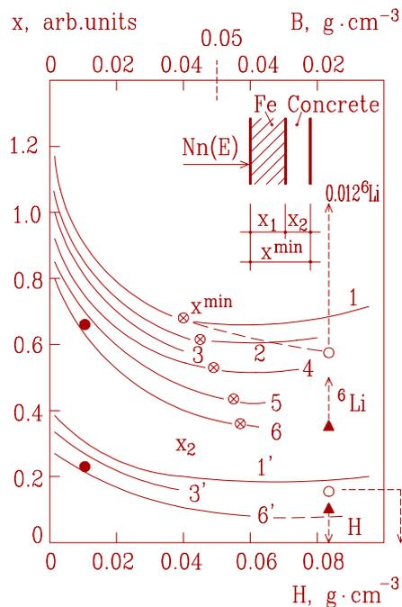
Figure 2: Shielding optimum. Density,  $\text{g}\cdot\text{cm}^{-3}$ : 1.2 (1, 1'); 1.8 (2); 2.3 (3, 3' - common); 2.6 (4); 3.2 (5); 3.6 (6, 6'); ● - 3.48 Gematit concrete, experimental data [9]; ▲ - 3.53 Polymerconcrete  ${}^6\text{Li}$  0.012  $\text{g}\cdot\text{cm}^{-3}$ ; ○ - 1.12 Polymerconcrete  ${}^6\text{Li}$  0.012  $\text{g}\cdot\text{cm}^{-3}$ ; ⊗ - Optimum  $X^{\text{min}}$ .
