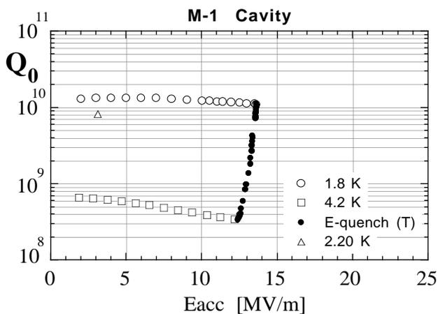
Figure: 2 The  $Q_0$  - Eacc plots in the test of the M-1 cavity.
