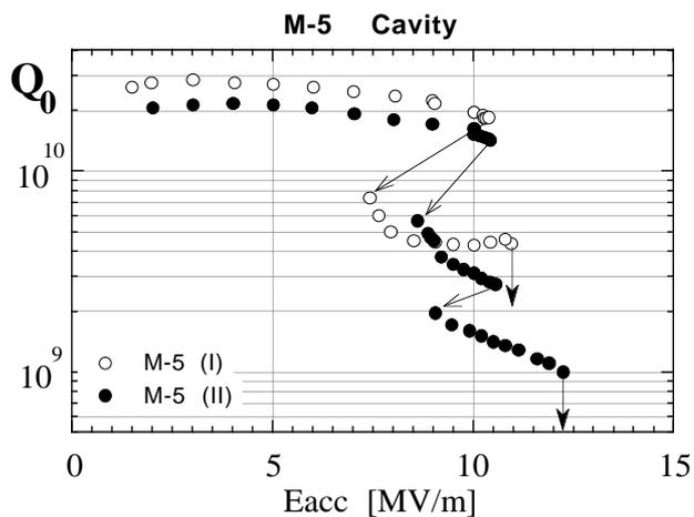
Figure: 6 The  $Q_0$  -  $E_{acc}$  plots (1.8 K) in the tests of the M-5 cavity, in which the stepped drop of the  $Q_0$  value was observed.
