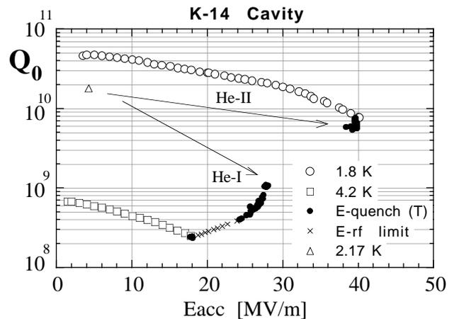
Figure: 4 The  $Q_0$  - Eacc plots in the test of the K-14 cavity.
