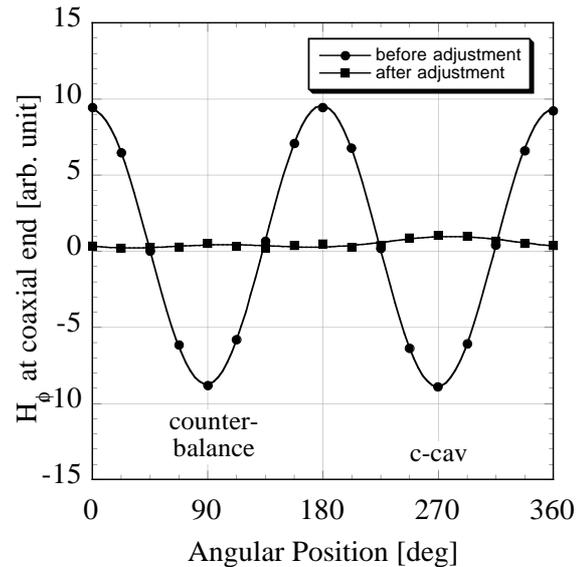
Fig. 4 Measured field that passed through the QCM choke in the middle of its adjusting stage (1/5 Al cold model).
