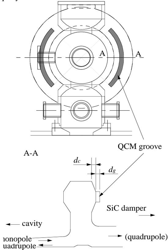
Fig. 2 QCM choke. Two grooves are on the side wall of the choke.
