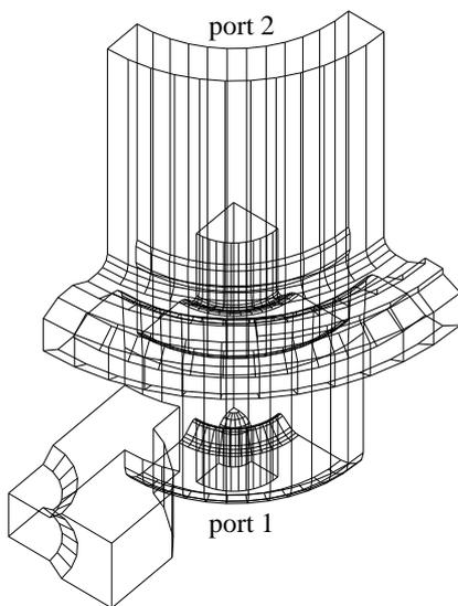
Fig. 3 HFSS model used in the design of the QCM choke.
