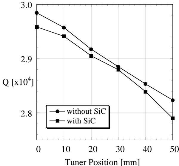
Fig. 5 Measured  $Q$  value of the first ARES high-power model with and without SiC damper in the chokemode cavity.
