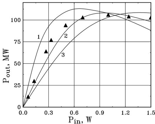
Figure 5: Amplitude characteristic of the klystron. Here  $\blacktriangle$  – experimental results and curves – theoretical calculations (1 –  $U = 1$  MV, 2 –  $U = 1.025$  MV, 3 –  $U = 1.05$  MV).
