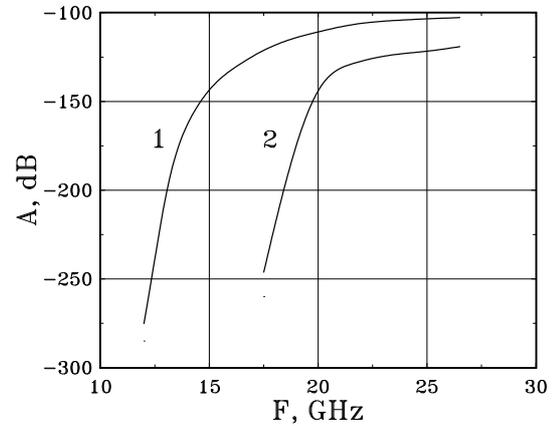
Figure 3: Integral frequency characteristic of the distributed suppression filter composed of ten RF absorbing insertions (1 –  $H_{11}$  mode and 2 –  $E_{01}$  mode).
