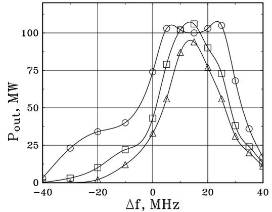
Figure 6: Frequency characteristic of the klystron. Here  $\triangle$  –  $P_{in} = 0.5$  W,  $\square$  –  $P_{in} = 1$  W and  $\circ$  –  $P_{in} = 2$  W ( $\Delta f = f - 14$  GHz).
