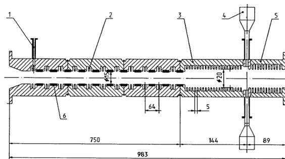
Figure 1: Layout of the klystron with RF absorbing insertions. Here (1) – input waveguide, (2) – resonators of buncher, (3) – output structure, (4) – RF load, (5) – RF filter for  $E_{01}$  mode, (6) – RF absorbing insertions (placed inside drift tubes).
