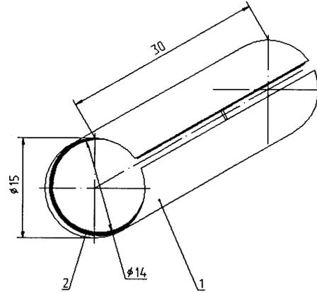
Figure 2: Scheme of RF absorbing insertions. Here (1) – metal foil, (2) – RF absorbing layer.
