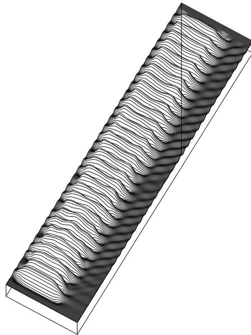
Figure 7: Wake field of a charge distribution that closely matches the E-z component of the fundamental mode
