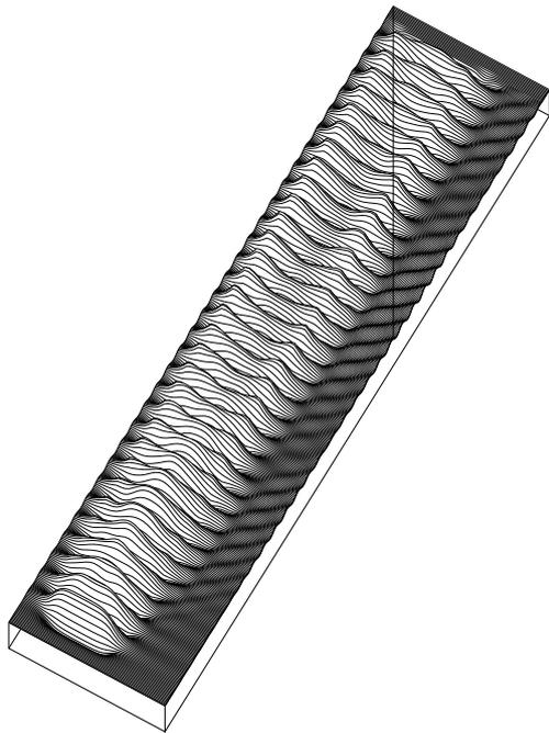
Figure 6: Wake field excited by a charge with rectangular density in x-direction, total width 1 cm
