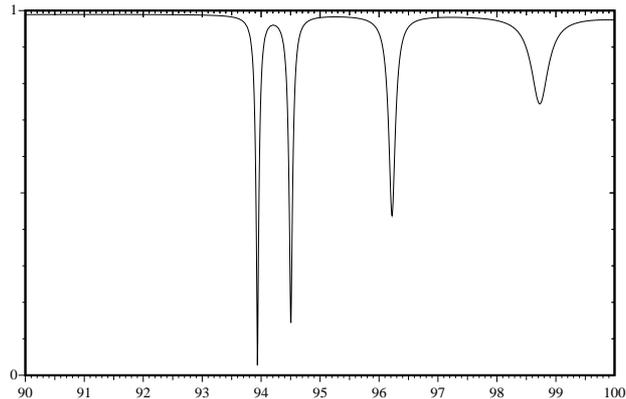
Figure 4: Reflection coefficient versus excitation frequency in GHz
