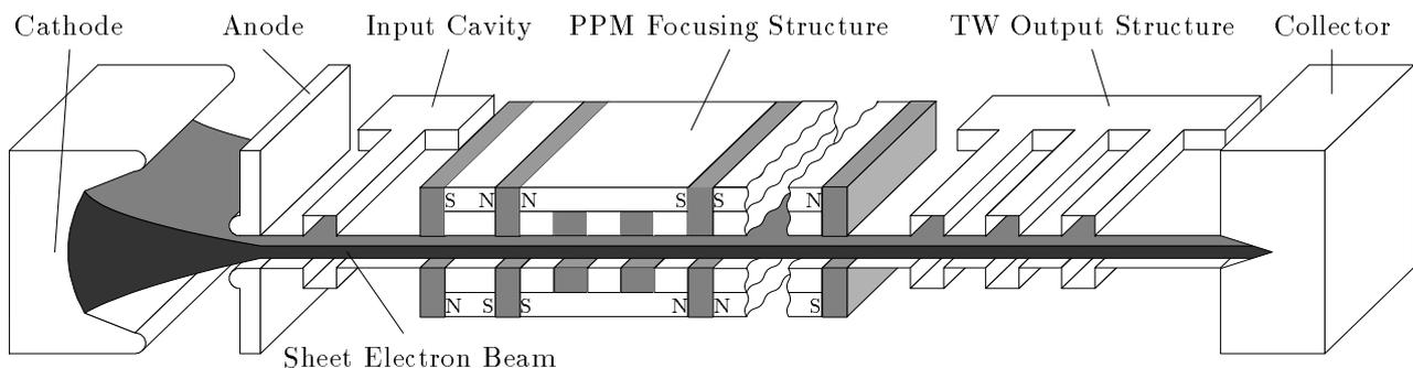
Figure 1: Schematic of the sheet beam klystron
