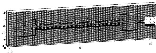
Figure 2: Coupled input cavity monochromatically excited, all dimensions in mm
