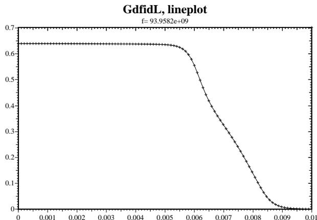
Figure 3: Longitudinal electric field over cavity width
