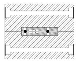
Figure 5: Cross-section of the RF structure with integrated cooling channels.
