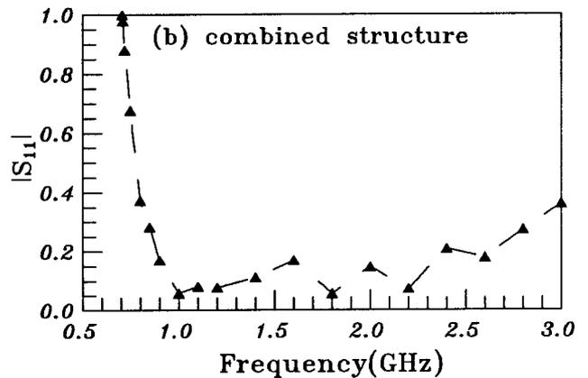
Fig. 2: (a) Reflection coefficient of the ridged circular waveguide and of the transformer part. (b) Reflection curve of the combined structure.
