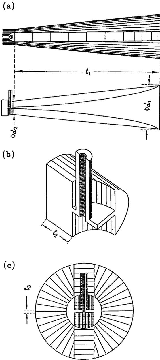
Fig. 1: Geometrical structure of the circular waveguide to coaxial transition,  $l_1 = 800$  mm,  $l_2 = 35$  mm,  $l_3 = 7$  mm,  $d_1 = 250$  mm and  $d_2 = 90$  mm.
