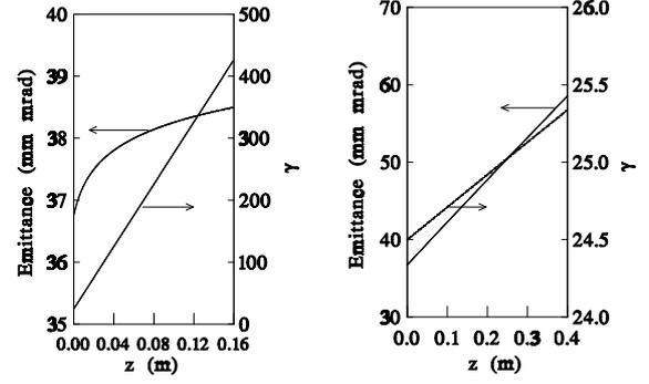
Figure 2: Emittance and energy variations along the interaction region when the resonance of the medium is in the optical range (left frame) and microwave range (right frame)
