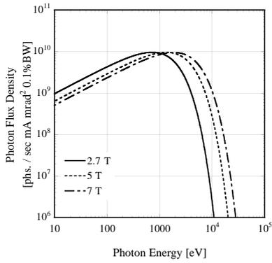
Figure 2. Spectrum from bending magnet, 5T wigglers and 7T wigglers.
