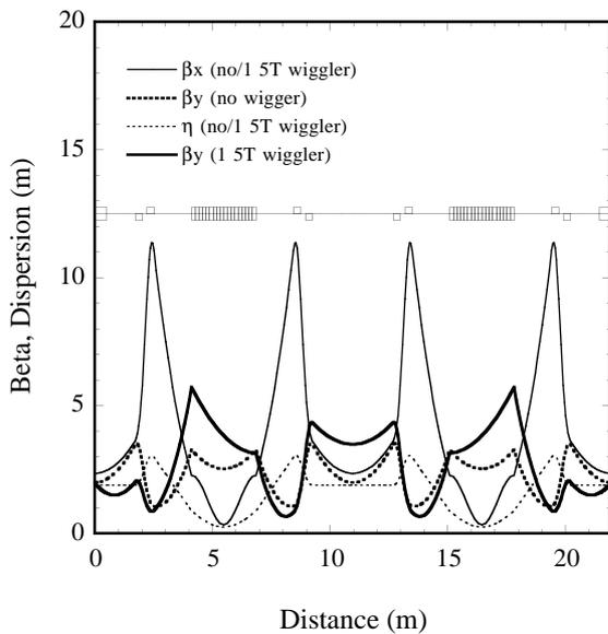
Figure 8. Lattice of no and single 5 T wiggler type.
