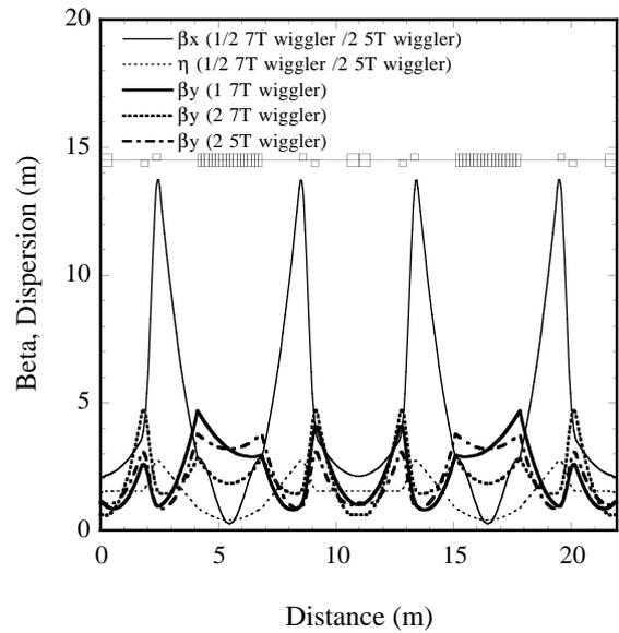
Figure 9. Lattice of single, double 7 T wigglers type and double 5 T wigglers type.
