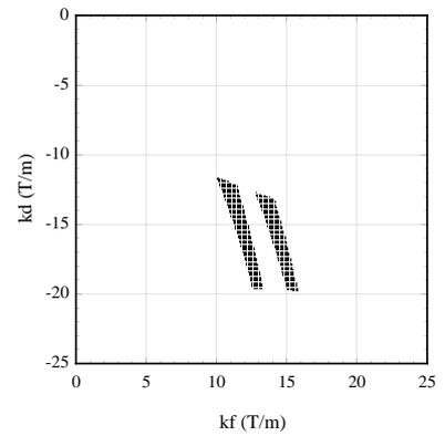
Figure 7. Double 7 T wiggler. Working point is  $k_f=11.1$ ,  $k_d=-12.5$  T/m.
