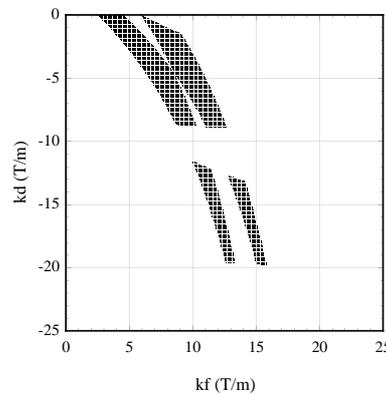
Figure 6. Double 5 T wiggler. Working point is  $k_f=11.1$ ,  $k_d=-12.5$  T/m.
