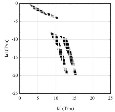
Figure 4. Single 5 T wiggler. Working point is  $k_f=10.2$  T/m,  $k_d=-10.0$  T/m.
