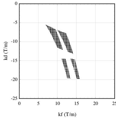
Figure 3. AURORA-2D no Insertion device. Working point is  $k_f=10.2$  T/m,  $k_d=-10.0$  T/m.
