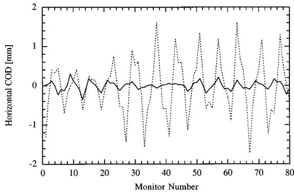
Figure 2: *Horizontal COD at every monitor location. The solid line is the case of the final setup, and the dotted line is the case of a random setup.*
