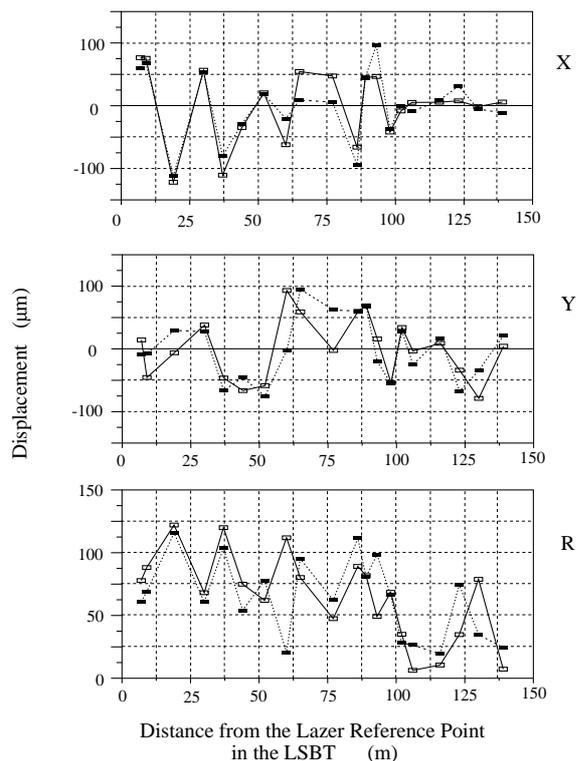
Figure 1: Displacement of 20 sets of magnets along the beamline. Three data were measured in series. X is horizontal, Y is vertical, and R is radial direction.
