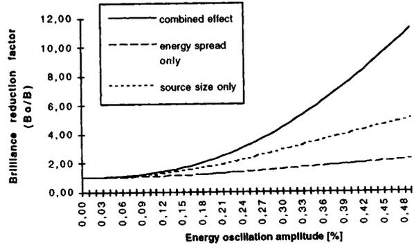
Fig. 3. Brilliance reduction due to bunch energy oscillations.
