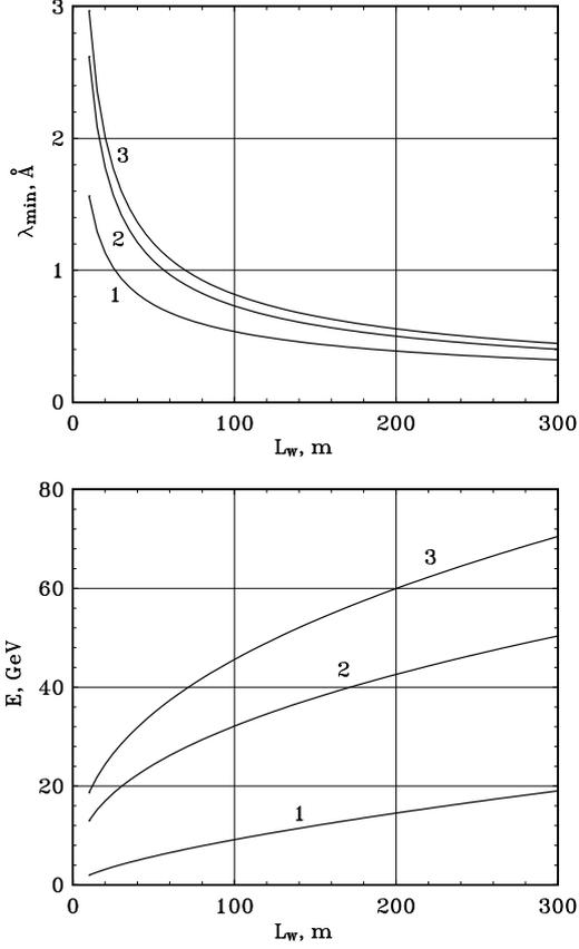
Figure 3: Minimal achievable photon wavelength in an FEL amplifier and corresponding energy of the electron beam versus the length of the undulator  $L_w$ . The curves 1, 2 and 3 correspond to values of the energy spread at the entrance of the undulator of 0 MeV, 3 MeV and 6 MeV, respectively. The normalized emittance is  $10^{-4}$  cm rad in all cases.
