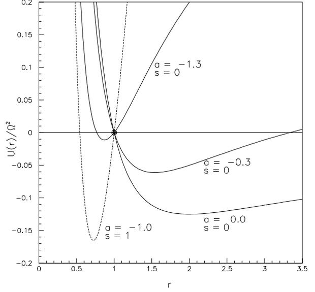
Figure 1: Effective potential  $U(r)$  for different types of induced voltage with RF off ( $s = 0$ ) and on ( $s = 1$ ).
