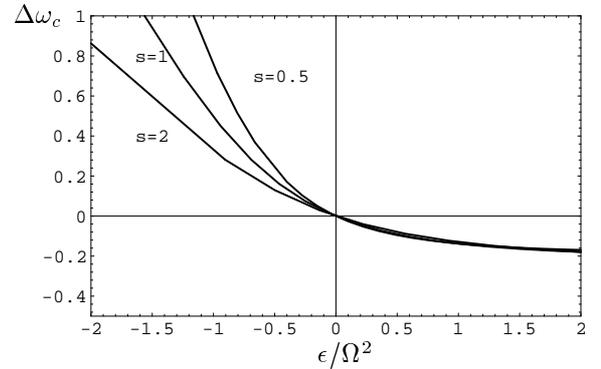
Figure 3: Coherent frequency of bunch shape oscillations  $\Delta\omega_c = (\omega_c - 2\omega_{s0})/\omega_{s0}$  as a function of intensity parameter  $\epsilon/\Omega^2$  for different values of RF voltage ( $s$ ).
