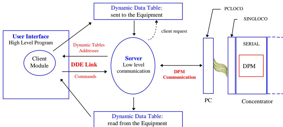
Figure 2 - Schematic layout of the high level software configuration.
