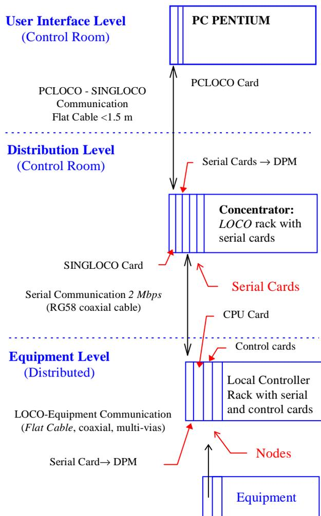
Figure 1 - Schematic layout of the Control System Structure
