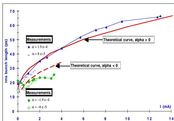
Figure: 2 Bunch Length versus Bunch Current
