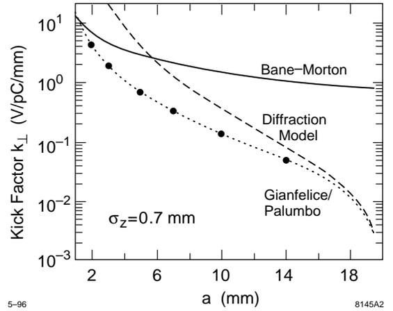
Figure 2: Transverse kick factor as a function of collimator half aperture  $a$ . The three curves correspond to three different analytical estimates, while the plotting symbols refer to the numerical calculations. A beam-pipe radius  $b$  of 2 cm is assumed.
