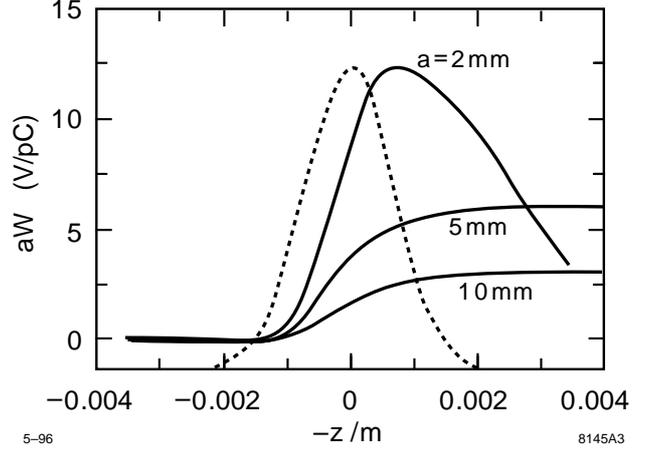
Figure 1: Dipole-wake function of a Gaussian bunch with  $\sigma_z = 0.7$  mm, as computed by MAFIA, for three different collimator half apertures  $a$ . The beam-pipe radius is  $b = 2$  cm; the beam profile is given by the dotted curve, with the head to the left.
