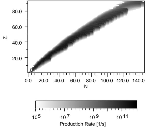
Fig. 1 Production rate of unstable nuclei at MUSES. Calculation assumes 100 $\mu\text{A}$  primary beam. The separator acceptance is 10mrad in angle and 1% in momentum. The production target is Be and its thickness is optimized so as to get maximum production rate. The kind of primary beam is also optimized among whole stable nuclei.
