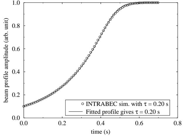
Figure 1: A computer simulation of electron cooling of  $^{20}\text{Ne}^{10+}$  in CELSIUS fitted by eq. (7).
