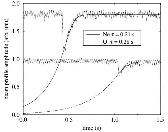
Figure 2: Measurements of  $^{20}\text{Ne}^{10+}$  and  $^{17}\text{O}^{8+}$  at injection energy together with theoretical fits.
