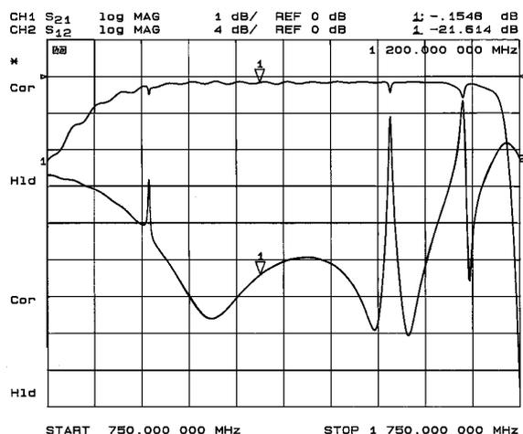
Figure 5: Custom circulator frequency response.
