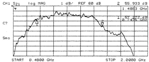
Fig. 2: Power amplifier frequency response
