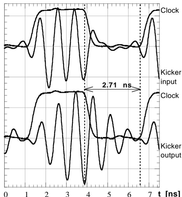
Fig. 7: Kicker input and output time-domain signals
