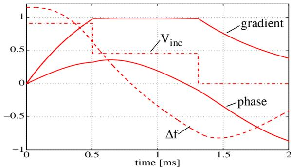
**Figure 1** : Open loop response. No beam. Incident power reduced to 25% at time of beam injection.
