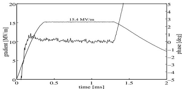
**Figure 3:** Analog feedback closed loop performance: cavity gradient and phase.
