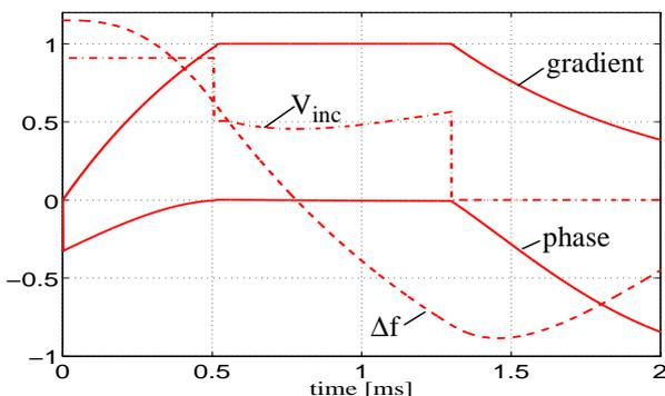
**Figure 2** : Closed loop response with simulated beam. Amplitude and phase are constant during beam acceleration. The forward power is time dependent due to time varying cavity detuning.
