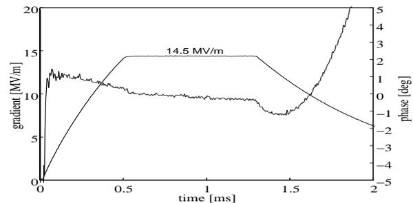
**Figure 4:** Digital feedback closed loop performance: cavity gradient and phase.
