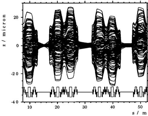
Figure 2: Simulated closed orbits with feedback using four magnets per straight section.
