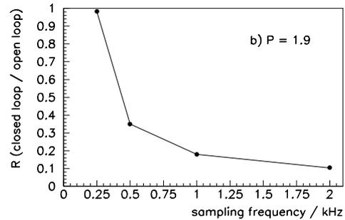
Figure 4: Feedback efficiency (defined in the text) as function of a) BPM error and b) sampling rate.
