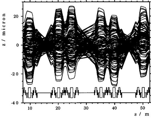
Figure 1: Simulated closed orbits without feedback.
