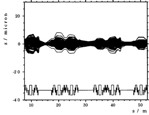
Figure 3: Simulated closed orbits with feedback using a scheme with two magnets per straight section.
