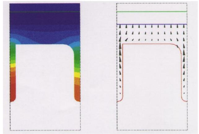
Figure 4: Temperature distribution and thermal gradient in a cut at one of the eight cooling channels. Only the upper half is shown. Compare also Fig. 1.
