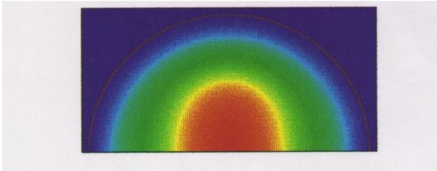
Figure 7: Temperature distribution in the ceramic pane of the rf-window.
