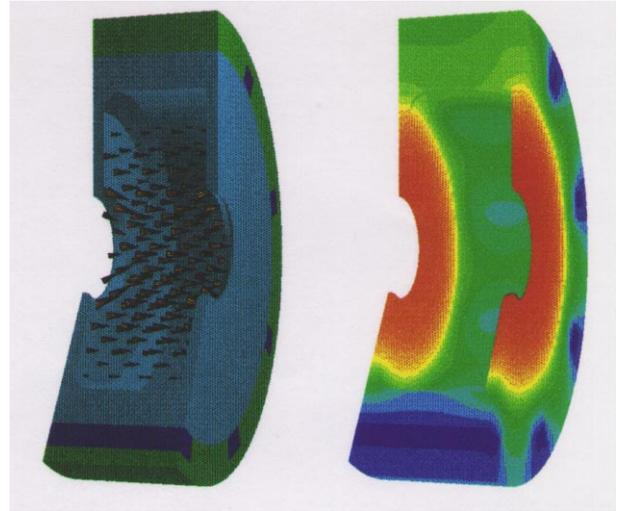
Figure 1: Vector plot of accelerating field and resulting temperature distribution in one of the 180 cells of the water-cooled SBLC-structure. Part of the structure is cut away to look inside.
