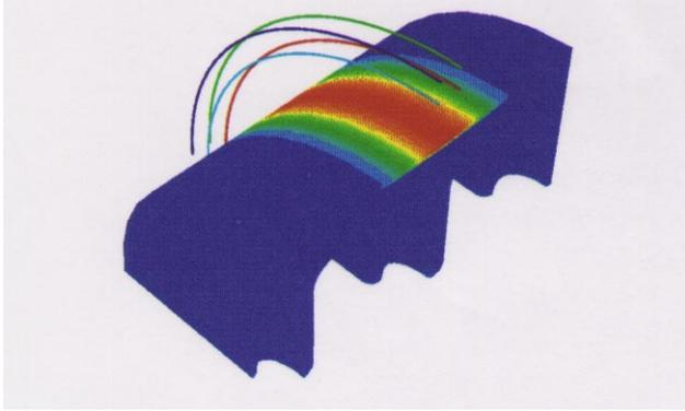
Figure 2: Energy density distribution produced by the driven coils in one quarter of the cylindrical structure.
