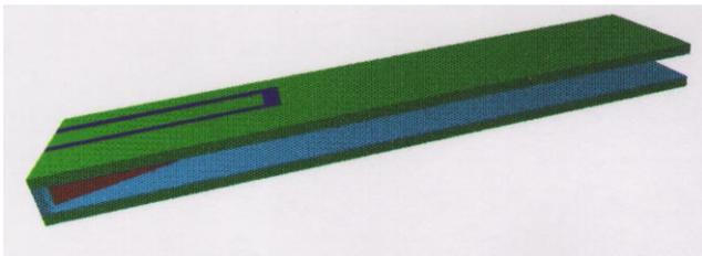
Figure 8: Geometry of a waveguide with load and attached cooling channel which can be seen on the outside.
