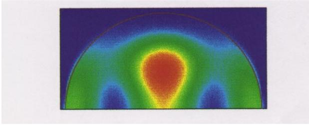
Figure 6: Energy density distribution in the ceramic pane of the rf-window.
