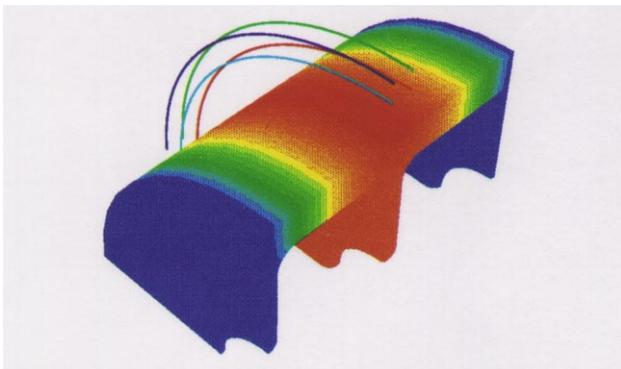
Figure 3: Temperature distribution: The area near the coils and the middle iris is heated.
