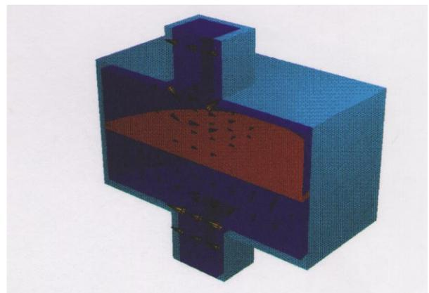
Figure 5: Vector plot of the electric field in an rf-window.
