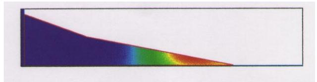
Figure 10: Temperature distribution in the lossy load.
