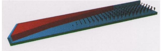
Figure 9: Vector plot of the electric field in a waveguide with load. The upper wall is cut away for this presentation.
