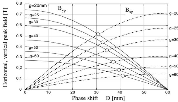
Figure 2 The horizontal and vertical peak fields on-axis as function of the phase shift  $D$ . Open circles are points of circular polarization.  $B_{yp}$  represents vertical peak field.
