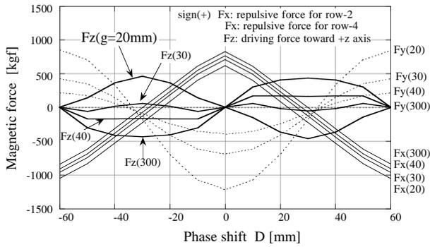
Figure 3 Magnetic force working on the magnet row-1.  $F_x$  is x-component of the magnetic force.
