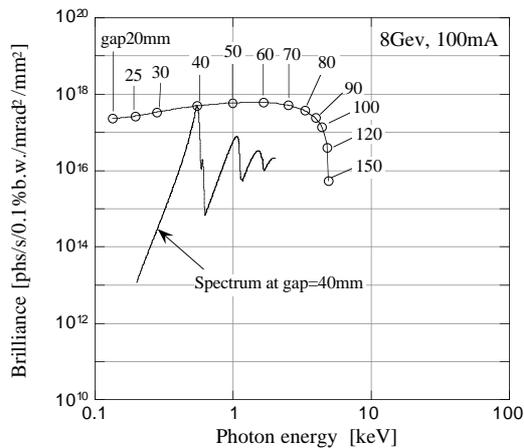
Figure 4 Brilliance of fundamental radiation as a function of gap distance at circular polarization mode.
